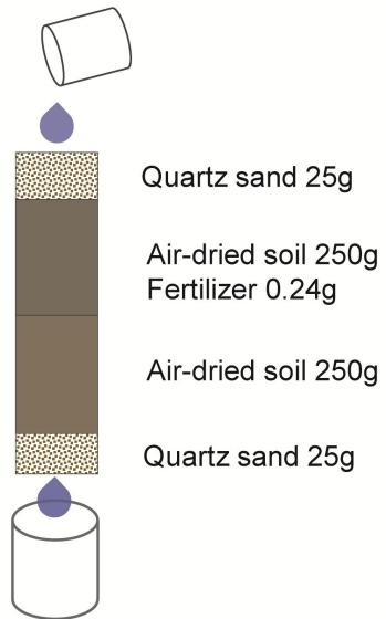
34 35 Figure S3 Simulation diagram of soil column leaching test. 36 Soil column leaching tube from top to bottom is 25g quartz sand, 250g air-dried soil and 37 0.24g fertilizer, 250g air-dried soil, 25g quartz sand.
