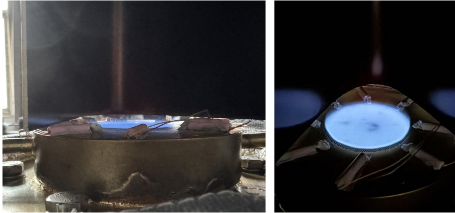
Figure 2 The planar flame on the burner plate for the methyl decanoate with \Phi = 1.0 at 373 K and 1 atm.
