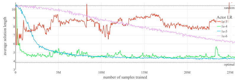
Figure 30: Performance throughout the training of four of Kool, Van Hoof, Welling's agents with different learning rates.
