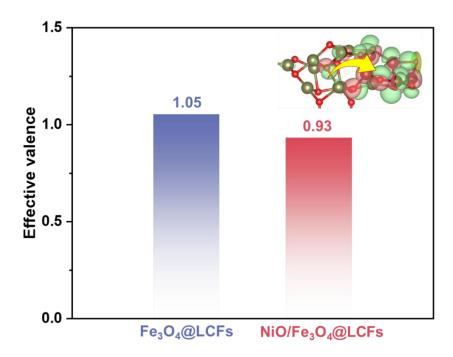
**Supplementary Fig. S4** Valence states of Fe atoms in Fe<sub>3</sub>O<sub>4</sub>@LCFs and NiO/Fe<sub>3</sub>O<sub>4</sub>@LCFs.
